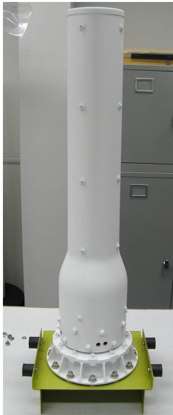
Figure 9 : SARAL/AltiKa UHF antenna
